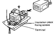
5) Attach the solid state color camera to the mounting angle of fan/heater unit using with supplied bolt and washer.
