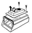
Attach the fan/heater unit to the housing mounting bracket using with supplied four screws and washers.
